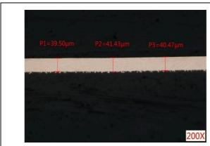
Fig.M01.9 Surface copper thickness (B-1)
