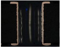
Fig.M015 The whole Surface copper thickness (A-1)
